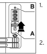
1. Set the combination to the factory default number. To test it, check whether the opener **A** can be pushed up. While setting the new combination leave the zip puller outside the lock.
